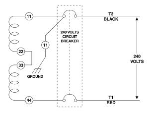
Do NOT connect loads in excess of circuit breaker ratings.
